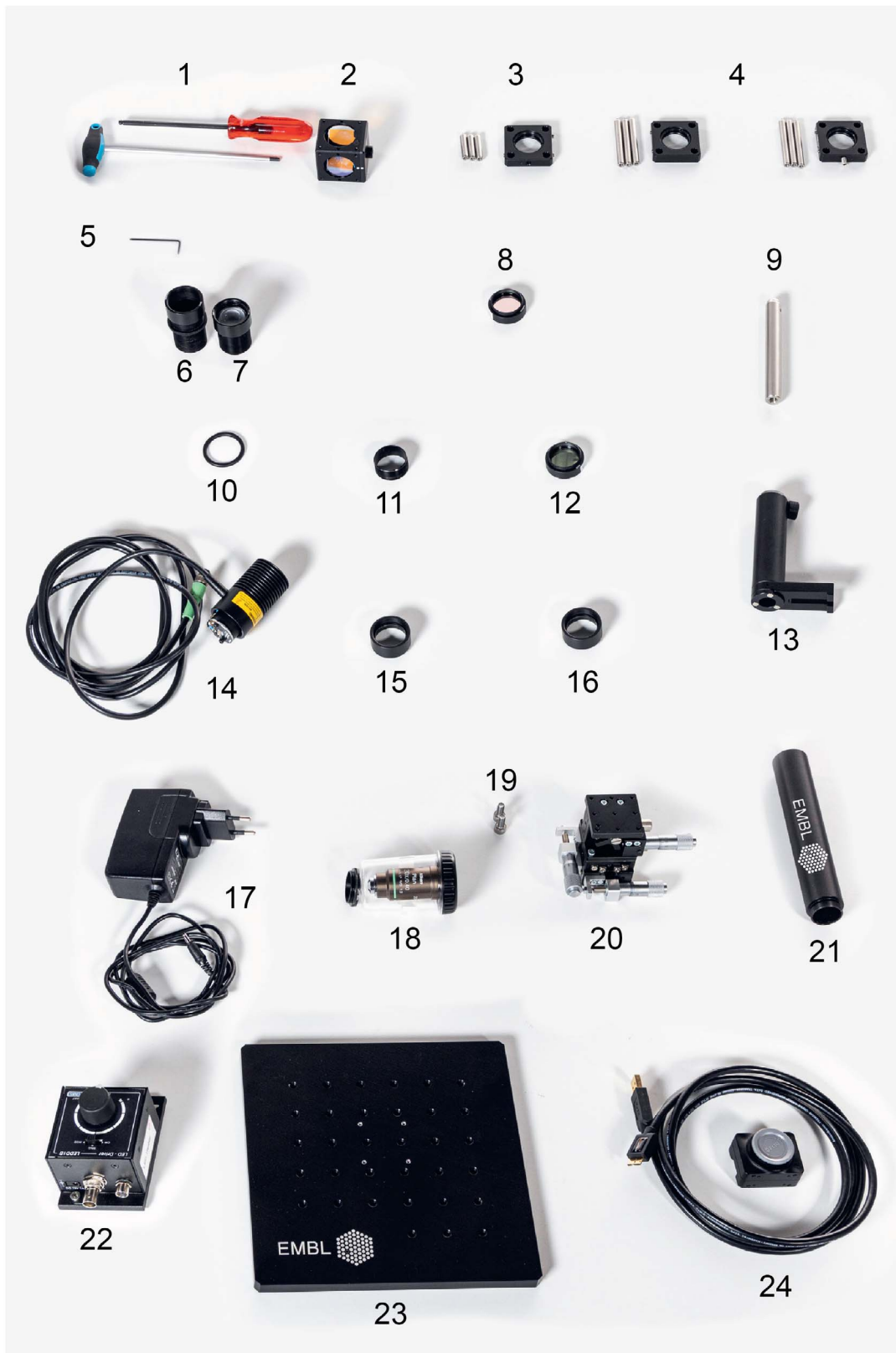
Fig 2. Components of the microscope building kit. (1) Screwdriver, (2) cage cube and dichroic mirror, (3, 4) cage plate and assembly rods, (5) Allen wrench, (6) adjustable lens tube, (7) collimator lens, (8) excitation filter, (9) post, (10) locking ring, (11) coupler, (12) emission filter, (13) post holder, (14) LED, (15, 16) tube lenses, (17) LED power supply, (18) objective lens and adaptor, (19) screws, (20) XYZ stage, (21) extension tube, (22) LED driver, (23) breadboard, (24) camera and connecting cable.
