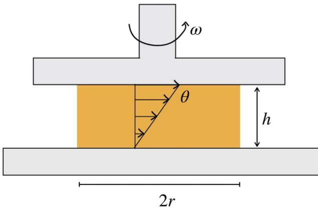
**Fig 2.** Schematic of a parallel-plate rheometer. The sample consists of a material in a circular disc of diameter  $2r$ , wedged between 2 plates, spaced a distance  $h$  apart. The bottom plate is fixed, and the top plate rotates at a frequency  $\omega$ , allowing the application of strain  $r\theta/h$ , where  $\theta$  is the amplitude of the angular displacement.
