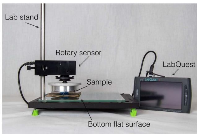
**Fig 4.** Design of the torsion rheometer. A photograph of the torsion rheometer device. The sample is cut into a circular disc and then placed on a flat surface. The rotary sensor is mounted on a lab stand and brought down in contact with the sample. LabQuest is connected to the rotary sensor to provide live angular displacement data over time.
