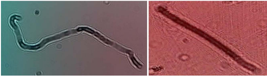
Fig 15. (Left) Cotton ball fibers are observed to have greater curvature and more kinks than (right) polyester fibers.
