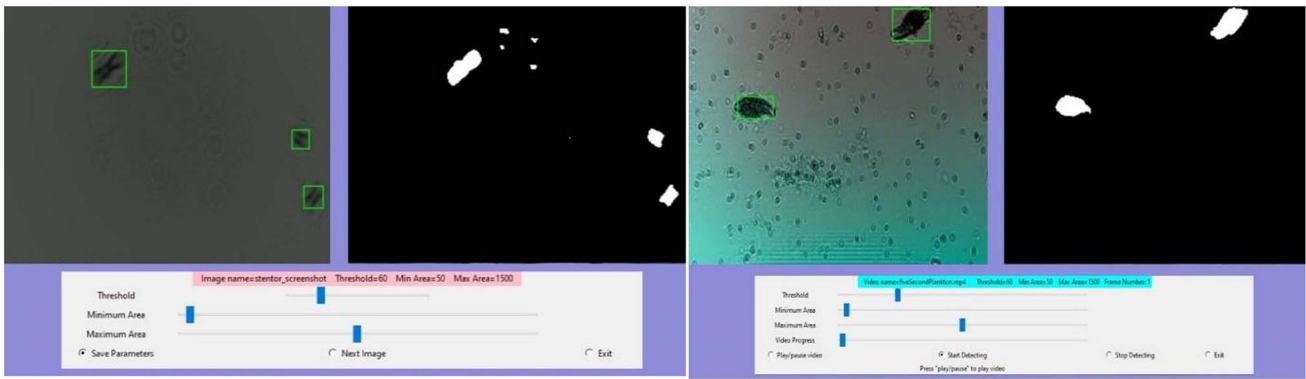
Fig 13. GUI for pipeline functions. (Left) Application to adjust detection parameters and label and save cropped images of objects. (Right) Application to adjust detection parameters to track selected objects in a video.
