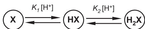
Fig 3. Diagram for an acid with 2 ionizable groups. The factors over the connecting branches relate the probability of each state to that of the preceding state.
