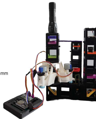
Fig 4. Examples of microscopes built by the students. (A1) Rendering of an upright dark-field microscope that uses a phone as the detector. (A2) Photo of the eventual microscope built by the students. (A3) An image of a microscopic ruler taken with this microscope for the technical report; the space between 2 long lines is 0.1 mm. (B1) Exploded rendering of an inverted bright-field microscope, which is motorized and uses a half mirror for dual detection by both an Arducam camera (STEP file used in the rendering from Allied Vision) and a phone. (B2) Photo of the eventual microscope built by the students. (B3) An image of a microscopic ruler taken with this microscope for the technical report; the space between 2 long lines is 0.1 mm. Pictures of the microscopes were taken with a Sony camera. Background removed with Adobe Express ( https://new.express.adobe.com/tools/remove-background ). Accessed October 2024). Renderings made with Blender (4.3 LTS; Blender Foundation, The Netherlands) and edited in Affinity Designer (Affinity Designer 2.6.0, Serif Ltd., UK).
